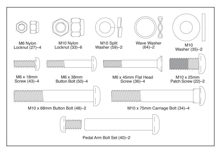
Identify the Front Stabilizer (10), which is narrower than the Rear Stabilizer (not shown). While another person lifts the front of the Frame (1), attach the Front Stabilizer with two M10 x 75mm Carriage Bolts (34) and two M10 Nylon Locknuts (33).
